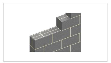
Walls can be tied together using metal ties or using masonry reinforcement, e.g., AMR-CJ masonry reinforcement.
