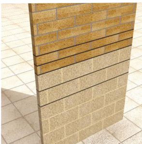
Figure 2.4 - Bed joint reinforced used to control movement between different walling materials.
